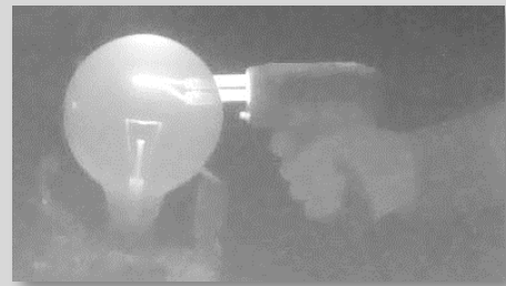
MWIR image using Phoenix Core (3-5µm) The filament and Soldering Iron are visible
